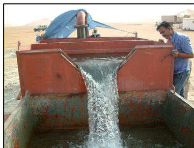
Open and shut-in pumping and aquifers tests were conducted on the artesian boreholes.
