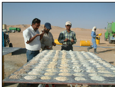
Identification of microfossils, to identify the contact between the U.UER (L. Eocene) and L.UER (Paleocene), was key to the successful completion of artesian boreholes.
