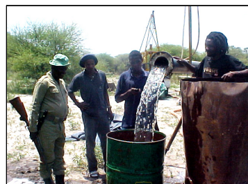
After drilling, pumping tests are conducted on all exploration boreholes to evaluate the potential of the aquifers and optimum yield. The Department of Wildlife provided protection to field crews in wildlife areas.
