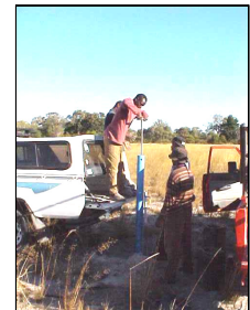
Piezometers were augured to measure the aquifer response to river recharge.
