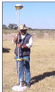
A high precision GPS survey at each borehole provided accurate locations and elevation of the boreholes.
